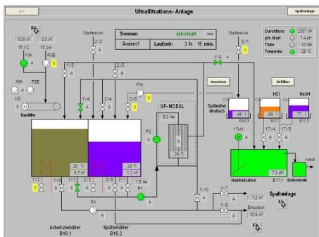
The oily rinsing water of a metal processing company is cleaned with an ultrafiltration plant (UF). If necessary the retained retentate is split with organic demulsifiers automatically with an **ARU** dosing control system.
