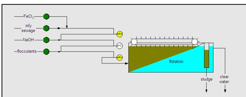
With the automation of the chemical dosage, the chemical costs have been significantly reduced. Optical control of the chemical dosage has increased the ease of operation and the operating reliability of the plant. **ARU** dosing controls are fully integrated into the process control system. In addition the demolition of a mixing reactor could reduce the space requirements of the plant significantly.
